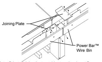
**Note:** Prior to joining the two tables together, insert Power Bar™ wire chase into one open end of wire bin. Center the wire chase in the opening of the two joined wire bins. Install #8-32 screws (BB) and nuts (CC) as shown. Do **not tighten.** Install the joining plates using #8-32 screws (BB) and nuts (CC). Align the wire chase and plates and tighten all hardware.
