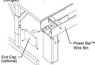
Slide wire chase into either end of the Power Bar™ wire bin (NOTE: remove joining panel supplied with wire bin, if installed). Install #8-32 screws (BB) and nuts (CC) as shown. Optional End Caps can be installed to close off both ends of the wire bin.
