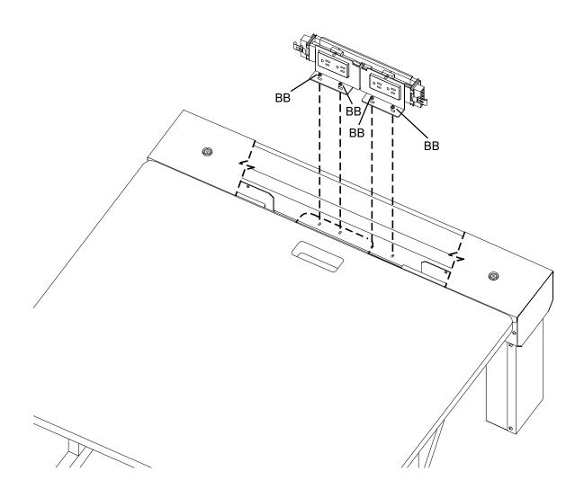
Partial interior view of Power Bar™ Wire Bin with optional End Caps and Wire Chase assembly shown.
