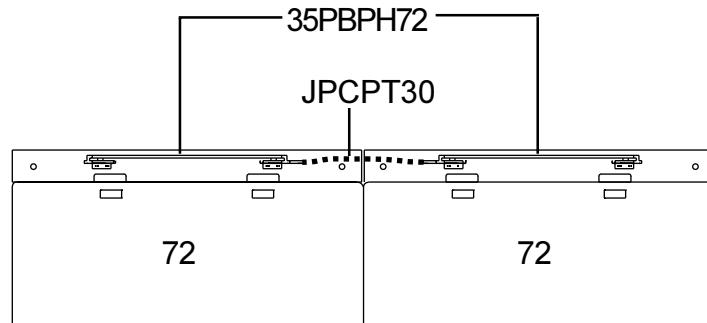
Use jumper LJUMP9696 (55 1/2" long) when joining a 24" Table Top Bridge between **any** combination of table to table connection.
