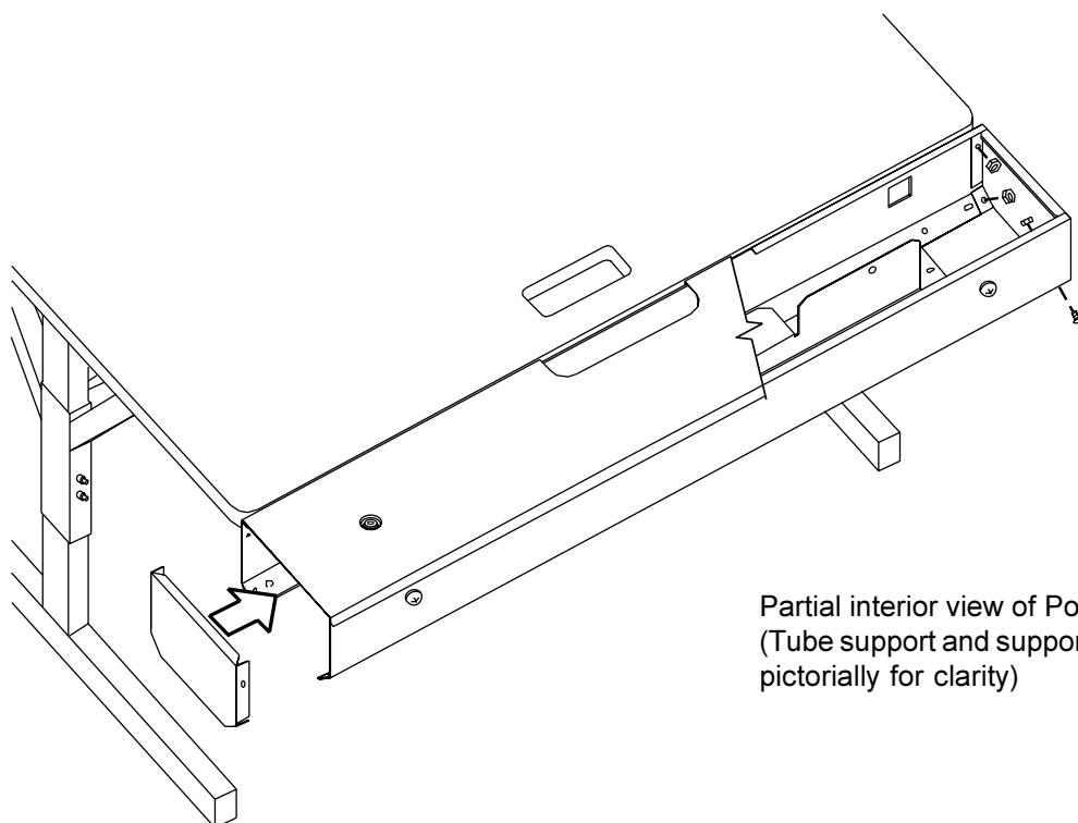
Install end caps on each end of the Power Bar™ wire bin as shown using #8-32 screws and nuts.
