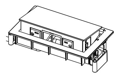
For desks including the Fluid Up Power Unit, mount the unit through the cut out and tighten from the underside using the thumb screws and locator slots. For further information, consult the assembly instructions supplied with the power unit.
