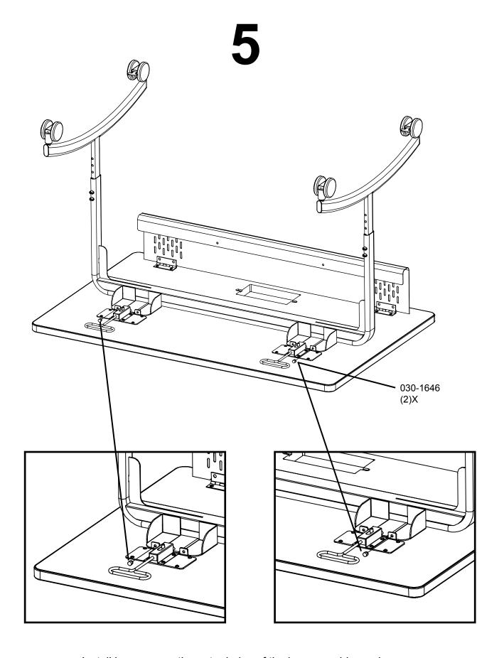
Install bumpers on the outer holes of the leg assembly as shown.
