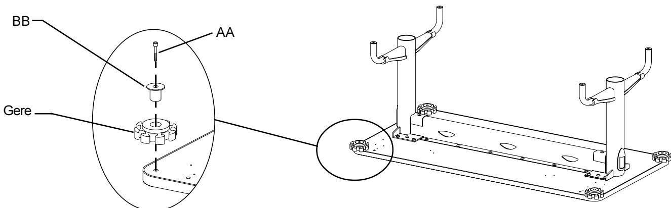
Install four sets of Gere Connecting Systems as follows. Insert 1/4-20 x 2 1/4" long socket head screw (AA) into the Table Connector Mount (BB). Slip the Table Connector Mount (with the screw) into the Gere as shown (be sure to orientate all Gere's the same way). Attach Gere assembly to each corner of the table using supplied Allen Wrench.
