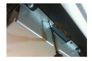
Assure that the brackets that mount the Power Island to the Main beam are fastened to the underside of the table using the 1' #12 screws AND that the Power Island is flush with the underside of the table.
