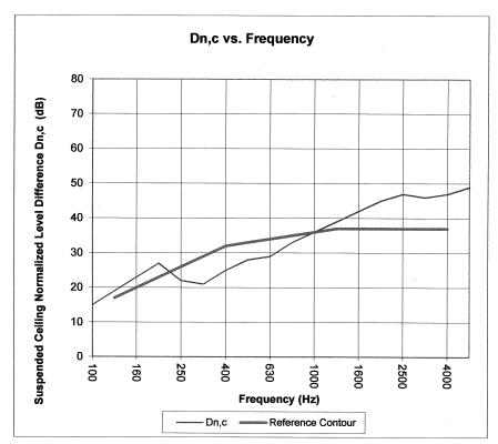
Dn,c = Normalized Ceiling Attenuation, dB Δ Dn,c = Uncertainty for 95% Confidence Level
