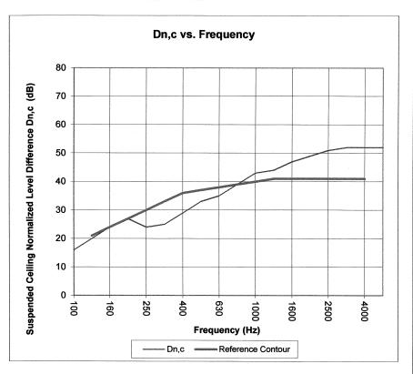
Dn,c = Normalized Ceiling Attenuation, dB  $\Delta$  Dn,c = Uncertainty for 95% Confidence Level
