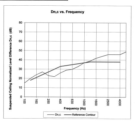
Dn,c = Normalized Ceiling Attenuation, dB ∆ Dn,c = Uncertainty for 95% Confidence Level
