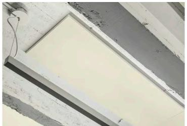
Akustika 25 Ceiling offers a surface-mounted acoustic solution that can softly fade into the background or create an unexpected pop of color and texture. 3mm Wool Design Felt is flush-mounted to one side of the substrate and achieves a 0.7 Noise Reduction Coefficient (NRC) rating. Available in 63 colors of 3mm Wool Design Felt, Akustika Ceiling is available with the Interlock Mounting System that allows for a quick and easy installation, even in an occupied space.
