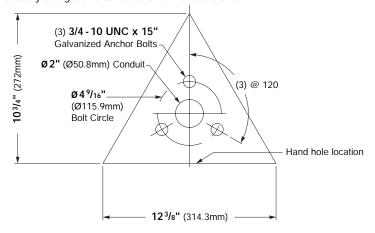
Note: Adequate drainage must be provided in concrete foundation or grout.
