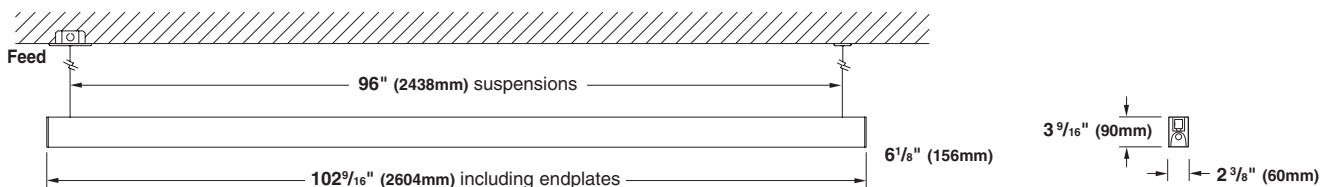
Typical Wall Mount - Top View (8' Nominal individual shown)
