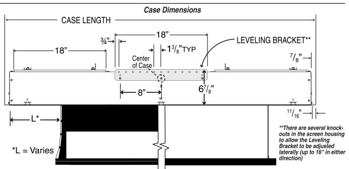
For ceiling cutout subtract 1½" from case length and width (measured from outer edge of flanges).
