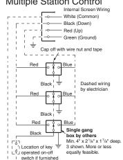
\*These wiring diagrams are for Access screens with motor on audience left (standard), and fabric unrolling from the back of the roller (standard).
