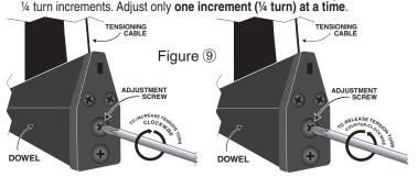
① If problem is not corrected, leave screen in position for 24 hours to allow surface material to stretch into position.
