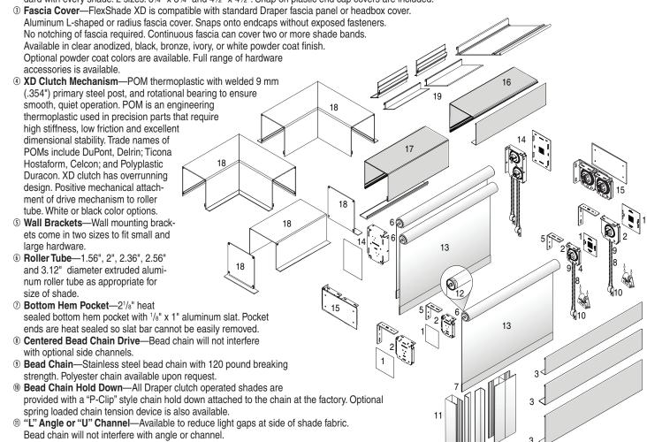
® Fabric Attachment—Shade fabric attached to aluminum roller tube with spline fabric attachment method. Allows for easy removal of fabric panel without removal of roller tube assembly.
