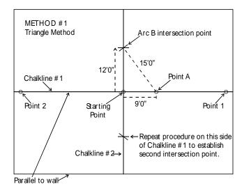
**Chalkline #1:** Regardless of method, chalkline one – also referred to as the "baseline" - is snapped roughly parallel to some architectural feature (outside wall, column line, etc.) and generally runs the longer dimension of the area. This is done by placing two and only two points on the floor as far apart as
