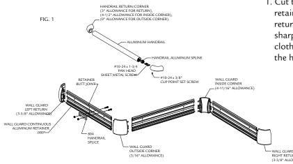
1. Cut the aluminum handrail top and aluminum retainer to the desired lengths leaving allowances for returns, outside corners and inside corners. Break sharp edges on aluminum handrail with fine emery cloth. Wall guard aluminum will be 3/8" shorter than the handrail top. See Figure 1.
