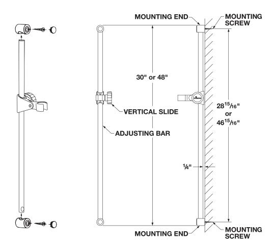
The Symmons hand spray adjusting bar is designed for easy installation and a neat, clean appearance.
