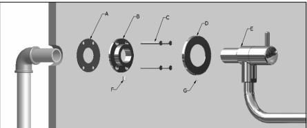
The adjustable flange allows for correct installation without the need for precise positioning of the internal pipe work. Therefore, the NPT connector should protrude from the wall / tile face 0 - 1/2".
