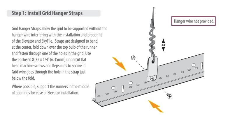
Note: Where possible, do not hang adjacent runners in the same 2' x 2', 60cm x 60cm, or 62.5cm x 62.5cm opening: installation of the Elevators and SkyTiles requires one open side above the grid into which they can be temporarily inserted before dropping down into the grid pocket.
