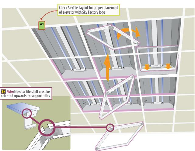
Elevator inserts diagonally up through the grid opening with the SkyTile shelf up. (Insertion is similar to inserting a standard acoustic ceiling tile.)
