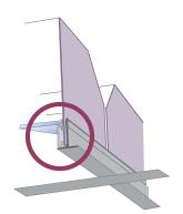
Support the Light-Box with 12 gauge (2.7mm) or comparable steel hanger wire using the slots located in each corner of the top of the fixture. Secure hanger wire to the ceiling according to national and local code.
