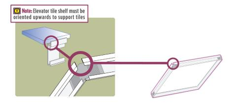
Elevator inserts diagonally up through the grid opening with the SkyTile shelf up. (Insertion is similar to inserting a standard acoustic ceiling tile.)
