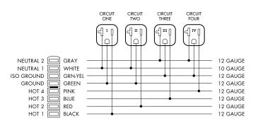
NOTE: The 4-circuit connection monument can utilize either of the above wiring schemes
