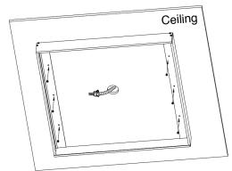
Mount the frame on the ceiling with screws (not included.)
