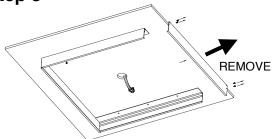
After mounting the frame on ceiling, **REMOVE** one side of the mounting frame.
