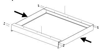
Assemble the mounting frame with the 8 screws (included).
