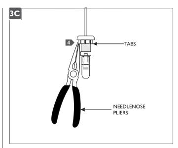
To adjust the glass holder (if necessary), bend the tabs in or out slightly with needlenose pliers.
