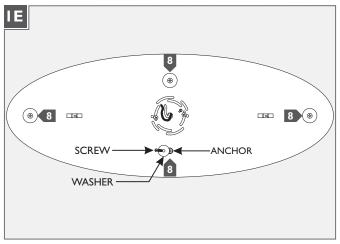
Secure the backplate to the anchors with a screw and washer on each of the four anchors.
