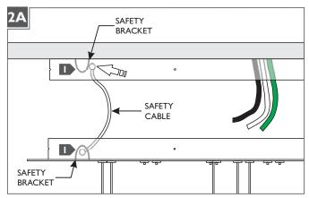
Hook a safety cable through the safety brackets on each end of the canopy and backplate.
