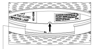
IMPORTANT NOTE: REST ALIGNMENT MARKERS WITHIN THE NOTCHES OF APERTURE AS SHOWN. THIS IS CRITICAL FOR PROPER ALIGNMENT.
