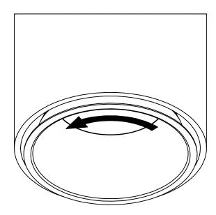
TWIST BOTTOM REFLECTOR 90° COUNTER-CLOCKWISE. ALTERNATIVELY, TWIST TOP SCREWS 90° CLOCKWISE
