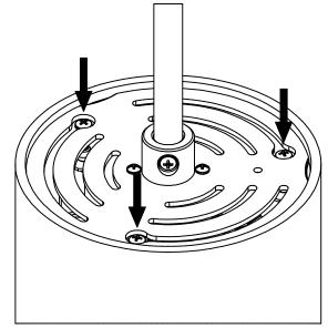
ALIGN SCREW HEADS WITH SLOT KEYHOLES AND, WHILE SUPPORTING BOTTOM REFLECTOR, REMOVE REFLECTOR ASSEMBLY FROM CYLINDER
