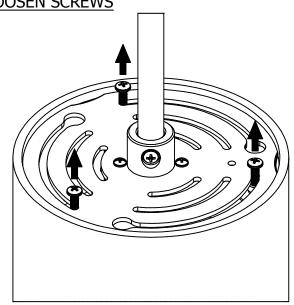
LOOSEN BUT DON'T REMOVE (3x) SCREWS ON TOP OF CYLINDER BY NO MORE THAN 1/2". BOTTOM REFLECTOR FLANGE WILL BE ACCESSIBLE FROM BOTTOM OF CYLINDER
