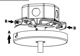
RAISE CANOPY AND TWIST INTO PLACE, THEN TIGHTEN (2x) CANOPY SCREWS
