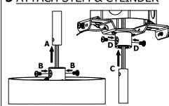
FEED WIRES THROUGH STEM, ALIGN HOLES, THEN FASTEN CYLINDER TO STEM WITH (2x) SCREWS. WITH CANOPY ON STEM, FEED WIRES THROUGH CROSSBAR, ALIGN HOLES, THEN FASTEN STEM TO CROSSBAR WITH (2x) SCREWS
