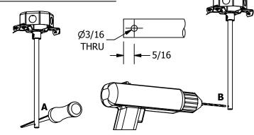
REVERSE STEPS 5, 4, & 3. CUT STEM TO DESIRED LENGTH AND DRILL A Ø3/16 HOLE THROUGH STEM 5/16" FROM BOTTOM. REPEAT STEPS 3-5
