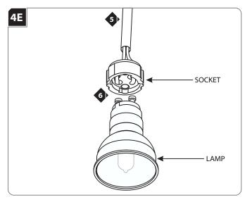
Use **ONLY** 120 Volt, **20** Watt GX10 Base MR16 Ceramic Metal Halide lamp.
