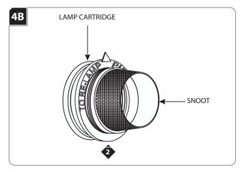
Unscrew the snoot from the lamp cartridge.
