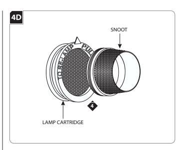
Replace and tighten the snoot completely to the lamp cartridge.
