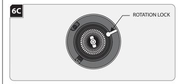
**NOTE:** Lamp housing can rotate 361° horizontally.
