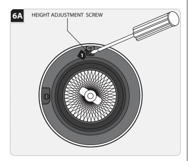
To adjust the height rotate the height adjustment screw. Adjust upward to minimize glare and flash on the trim or downward for maximum light output and efficiency.
