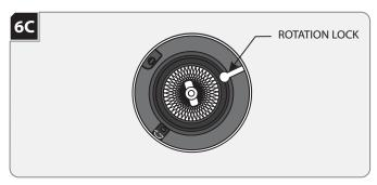
**NOTE:** Lamp housing can rotate 361° horizontally.
