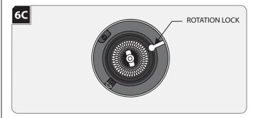
**NOTE:** Lamp housing can rotate 361° horizontally.
