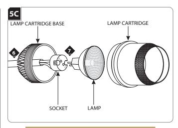
Use **MAX 50** Watt Type MR16 Halogen Lamp.
