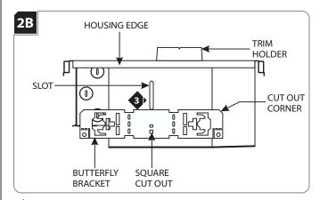
Line up the square cut out section of the butterfly bracket with the housing slot. Make sure the cut out corner of the butterfly bracket is against the housing edge.
