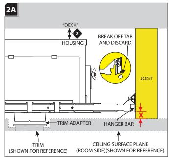
For a ceiling thickness between 3/8" and 1-1/2", use the provided dimensions or equation to determine the distance (X dimension) between the bottom of the hanger bar and the bottom of the joist.
