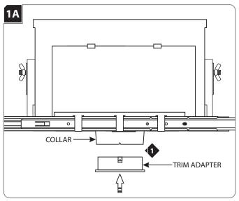
Install the trim adapter into the housing collar (trim holder) **PRIOR** to ceiling installation.
