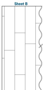
**Diagram 2** - Stagger the two sheets so that plank ends do not line up. This is indicated in yellow highlighting. Both edges of the sheet have a **narrow edge which needs to be trimmed** to leave behind a full plank. Overlap sheet B over sheet A as indicated below and cut in the joint (indicated by the red line), cutting both sheets so that the join runs down the edge of the plank.
