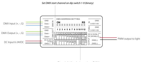
Dip switch 10 on (up) to activate DMX input
