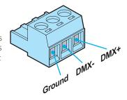
Insert the terminal block into the corresponding front panel socket and ensure that it fully clicks into place.
