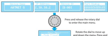
2 Turn the rotary dial clockwise/counterclockwise to move the highlight down/up the list of options, respectively.
