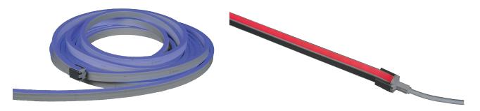
**Flex Tube RGB** is a color chaining, outdoor rated, flexible LED tube. It features a bend diameter of as little as 5", can be cut to length every 4", and features an IP68, submersible rating, suitable for any exterior application. It is sold in spools of 32' (10m), and is controlled via DMX-512.
