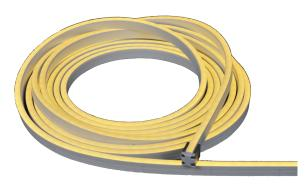
**Flex Tube SC** is a single color, outdoor rated, flexible LED tube. It features a bend diameter of as little as 5", can be cut to length every 4", and features an IP68, submersible rating, suitable for any exterior application. It is sold in spools of 32' (10m), and is, impact, UV, and saltwater resistant.
