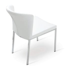
Capri Chrome is a contemporary dining chair with a comfortable upholstered seat and backrest on chrome plated steel legs. The seat has a steel structure with "S" shape springs for extra flexibility and strength. This steel frame is moulded by injecting polyurethane foam. Capri Sled is suitable for both residential and commercial use.
