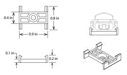
18" maximum recommended spacing between mounting clips.
