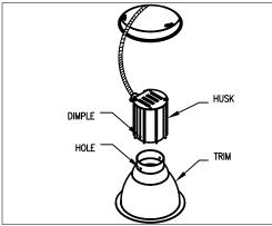
4.) ALIGN THE DIMPLE ON THE HUSK WITH THE HOLES IN THE REFLECTOR AND SNAP TOGETHER. SOCKET POSITION CAN BE RAISED OR LOWERED BY SQUEEZING THE SOCKET SPRING.
