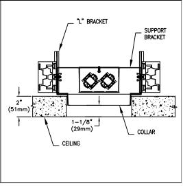
1.) REMOVE SUPPORT BRACKET AND SOCKET WRAPPER BY REMOVING WINGNUTS.
