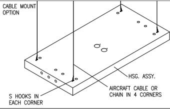
SURFACE MOUNT WITH (4) 1/4 20 SCREWS AND WASHERS TO A REINFORCED CEILING
