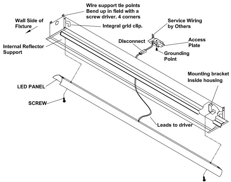
NOTE:Remove the LED panel to gain access to the driver for servicing.
