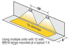
MR16 lamps mounted at a typical 7.5' delivers 30' center-center spacing on a 6' wide egress path.
