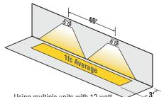
Using multiple units with 12 watt MR16 lamps mounted at a typical 7.5' delivers 40' center-to-center spacing on a 3' wide egress path.
