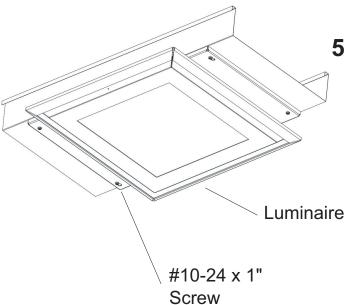
Leaving Tether attached, lift Luminaire up through the Collar. Position Luminaire over Mounting Bracket. Secure Luminaire with (4) #10-24 x 1" screws and tighten. (Note keyhole slots on opposite corners).
