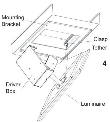
Using Clasp on the end of the Tether, attach Luminaire to Mounting Bracket through rectangular hole. Allow Luminaire to hang by Tether for wiring. Run supply wiring to box bottom. NOTE: K.O.'s are 1/2" conduit size. Make all primary wire connections. Flip Driver Box Cover top closed. Ensure all wiring is inside box and that no wires are pinched. Make sure wire tie keeps wires together to prevent pinching! Secure cover to box bottom with side screw.
