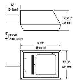
**HOUSING** - Radiused, rectangular shaped, die-formed aluminum. All hardware is stainless steel or electro-zinc plated steel.
