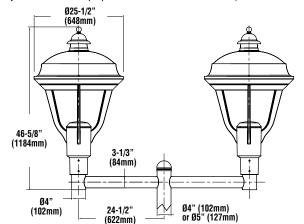
Post Top with BK MPT BO (x2) Mounts to 4" or 5" Dia. D180 Bolt-on Pole (select 3" reduced drilling pattern)
