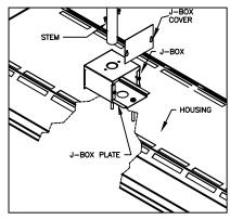
MONOPOINT J-BOX ASSEMBLY ONLY REMOVE J-BOX COVER AND MOUNT PLATE TO FIXTURE. THEN ATTACH SINGLE 3/4" IP STEM (ORDERED SEPARATELY). SLIDE HOUSING INTO PLACE INSIDE J-BOX AND MAKE WIRE CONNECTIONS. REPLACE J-BOX COVFR.
