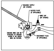
PULL BUILDING SUPPLY LEADS INTO HOUSING THROUGH THE ACCESS PLATE OR PIPE STEM. MAKE WIRE CONNECTIONS AS SHOWN. REPLACE ACCESS PLATE IF NECESSARY.
