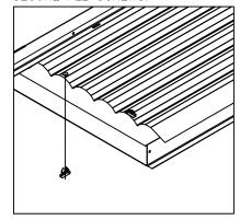
TO ACCESS DRIVER REMOVE LED PANEL BY ROTATING THE (4) 1/4 TURN FASTENERS 90°. THEN REMOVE DRIVER COVER BY REMOVING FOUR(4) SCREWS
