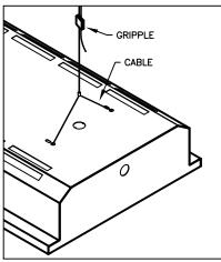
GRIPPLE ASSEMBLY ONLY. MOUNT THE FIXTURE BY FEEDING CABLE THRU GRIPPLE. ADJUST HEIGHT.
