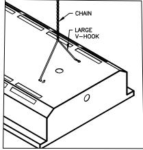
CHAIN ASSEMBLY ONLY. MOUNT THE FIXTURE BY USING THE LARGE V-HOOK AND CHAIN KIT. ADJUST HEIGHT.
