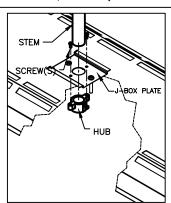
**HUB ASSEMBLY ONLY.** REMOVE REFLECTOR & DRIVER COVER TO MOUNT HUB TO INSIDE OF FIXTURE AND ATTACH TO SINGLE 3/4" IP STEM (ORDERED SEPARATELY). SECURE ALL SCREWS.
