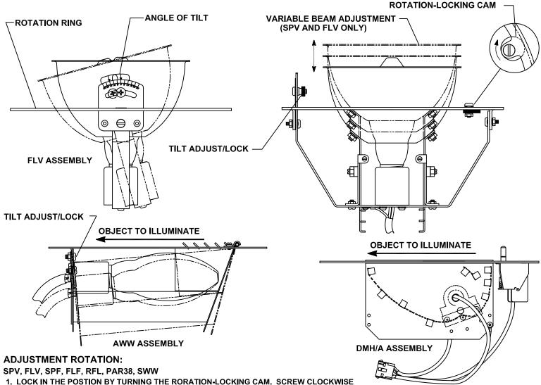
LOCK IN THE POSTION BY TURNING THE RORATION-LOCKING CAM. SCREW CLOCKWISE UNTIL IT ENGAGES THE INSIDE OF THE HOUSING.
