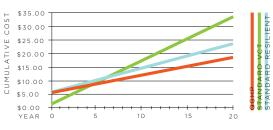
Break Even on Product and Maintenance Cost Difference Between: VCT VS. QGHP = 3 YEARS STANDARD RESILIENT VS. QGHP = 1 YEAR
