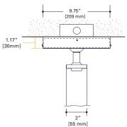
AC - Adjustable Sloped Adapter for surface junction box
