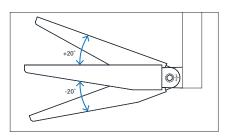
**RM** - Optional rigid knuckle mount for downward facing, fixed applications. Available in standard optic orientation only.
