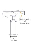
AR - Adjustable Sloped Adapter for recessed junction box
