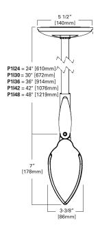
is standard, constructed of impactresistant, U.V. stabilized virgin acrylic to prevent discoloration.
