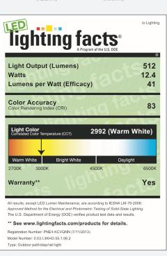
Label references 36" luxrail fixture with a 55° beam spread in High Output 3000K. Lighting Facts for additional beam spreads and light output levels may be obtained from io Lighting.
