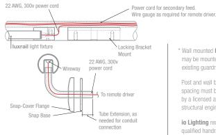
\* Wall mounted luxrail may be mounted to new or existing guardrail (by others).
